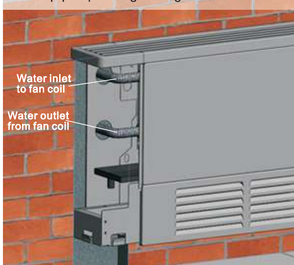
Water pipes passing through the wall
